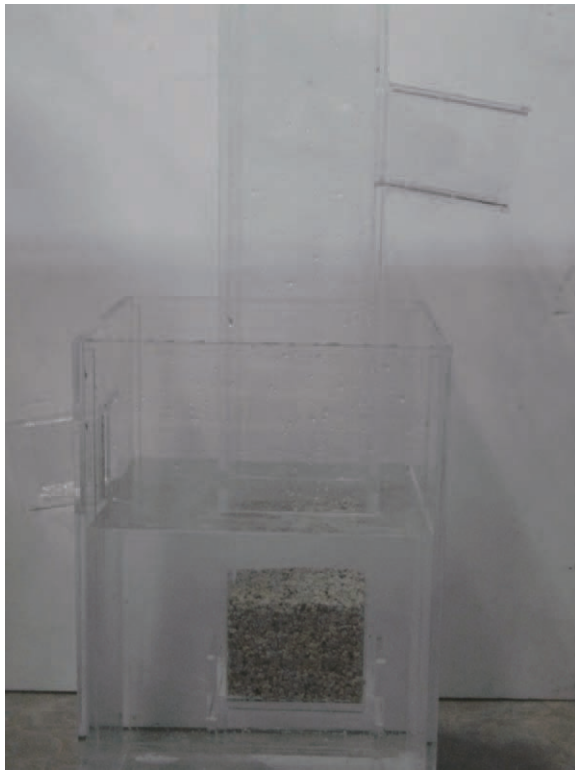
Figure 1 Water permeability test apparatus. [Color figure can be viewed in the online issue, which is available at wileyonlinelibrary.com .]
